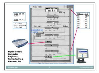
Five registers have three control inputs: LD (load), INR (increment) and CLR (clear). Two registers have only a LD input. (10)
