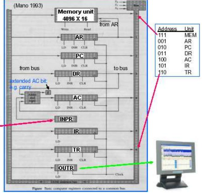
Five registers have three control inputs: LD (load), INR (increment) and CLR (clear). Two registers have only a LD input.
