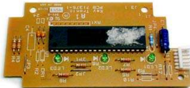
Microprocessor & Controller Circuitry of Keyboard
